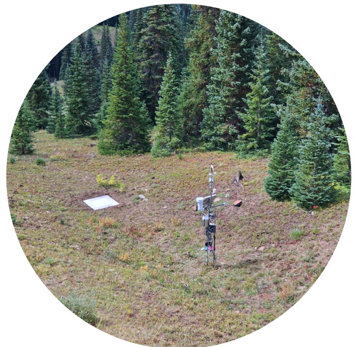
The installed snow pillow and Castle Creek station viewed from upslope (below). Image Credit: Asa DeHaan.
