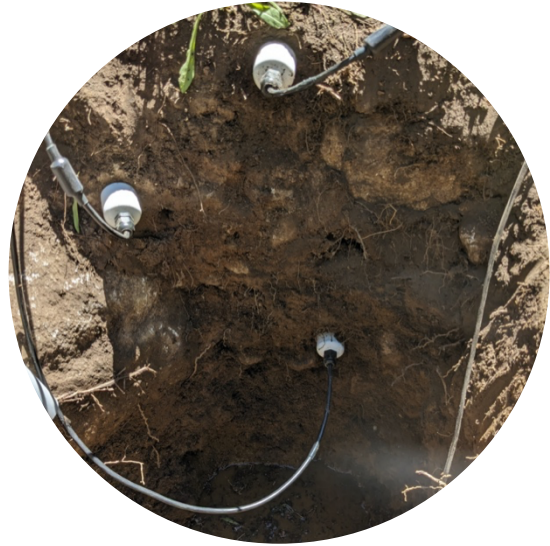
Soil moisture sensors inserted at 2, 8, and 20in in the pit at the Chapman SNOTEL site. The rocky soil profile is visible, as is the water table appearing at ~38in down. Image Credit: Asa DeHaan.
