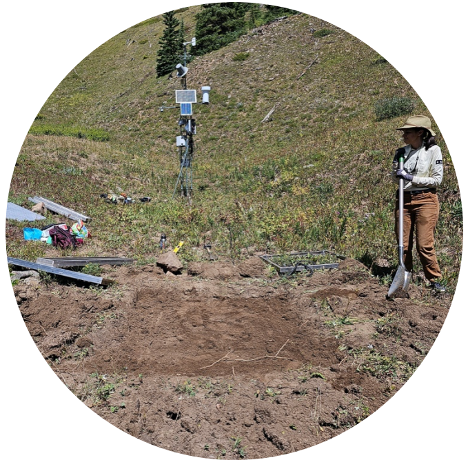
Elise Osenga (AGCI) prepares the ground to install a snow pillow at Castle Creek (above). Image Credit: Asa DeHaan.
